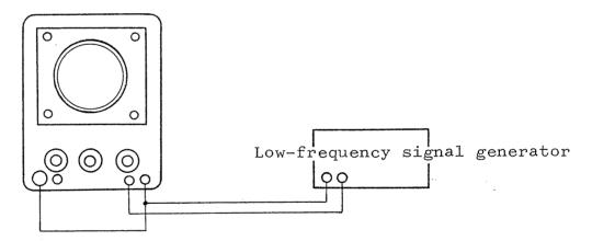
Adjust the SENSITIVITY switch, and VARIABLE AND AMPLITUDE knobs so that a figure of appropriate size is traced on the screen as shown below. Vary the frequency of the low-frequency signal generator, then a loop figure will be formed as shown at a frequency of several tens of kiloherz.
