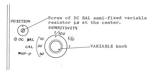
Adjustment of horizontal axis DC balance
