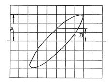
The intrinsic phase difference can be obtained as follows: Set the horizontal and vertical amplitudes of the loop figure to the scale as shown above, read values A and B, and calculate the phase difference angle by using the following formula:
